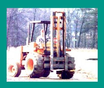
This operator is keeping his forks close to the ground while negotiating rough terrain.
